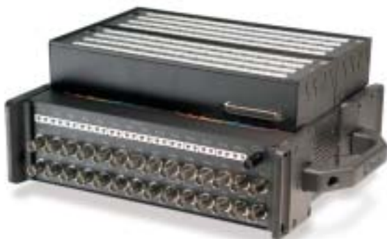
DaqBook/2020 system plus 112 additional channels of thermocouple input (DBK90)
