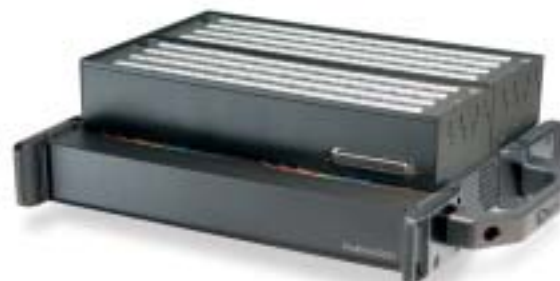
DaqBook/2001 plus 112 channels of thermocouple input (DBK90)
